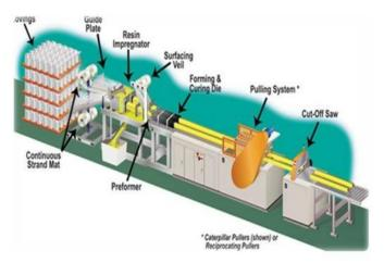
Figure 1: Process Of GFRP Structural Sections.
