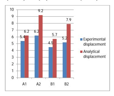
The results obtained from both the experimental programme and analytical studies are in good agreement. The modes of failure is also same in both experimental and analytical studies. The Graphs 1 and 2 shows the comparison of analytical and experimental displacement and stress values.
